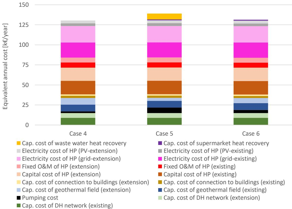
Figure 11: Composition of the equivalent annual cost of the extended DH system in case of 1: geothermal field only (see previous subsection); 2: recovery of waste heat from both the supermarket and the waste water pipe; 3: recovery of waste heat only from the supermarket.
