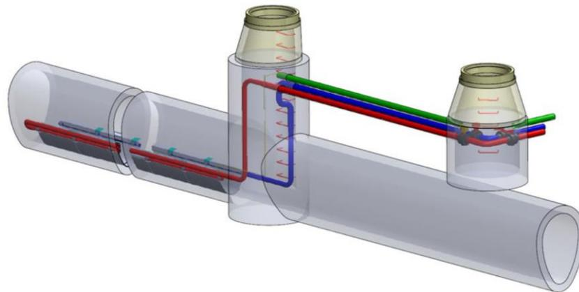
*Figure 8. Principle of thermal activation of waste water tubs. A special heat exchanger is installed within the waste water duct (large grey pipe in the figure). Supply and return pipes (red and blue pipes in the figure) of the recovery circuit connected it to the district heating network.*
