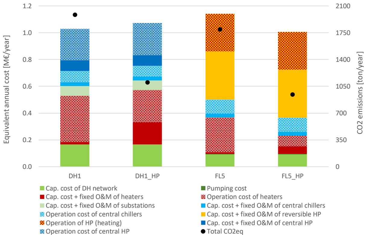
Figure 18: Composition of the equivalent annual cost and CO<sub>2</sub> emissions in the scenarios DH1\_HP and FL5\_HP using a centralized heat pump as central heater. The cases DH1 and FL5 using gas boilers are also shown as comparison.
