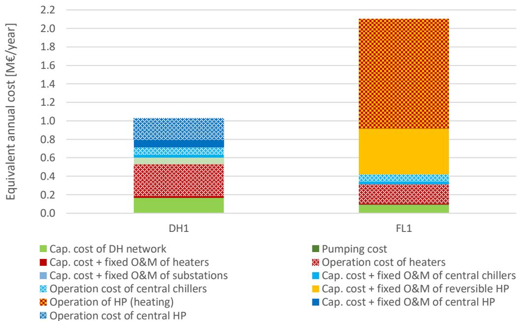
Figure 16: Composition of the equivalent annual cost in case of conventional DH (DH1) and FLEXYNETS (FL1).
