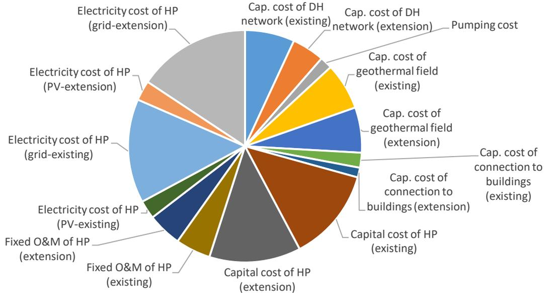
Figure 9: Composition of the equivalent annual cost of the low-depth geothermal DH system in the extended DH system (geothermal field only).
