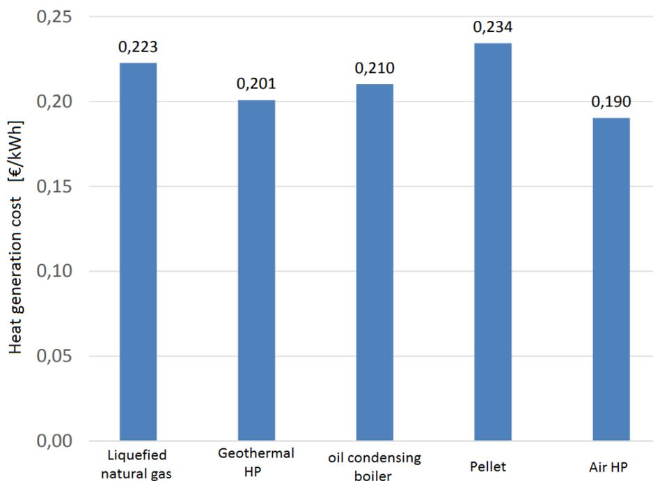
Figure 6: Heat generation cost for different heating technologies in Germany, 2014 (Brennenstuhl, 2017).
