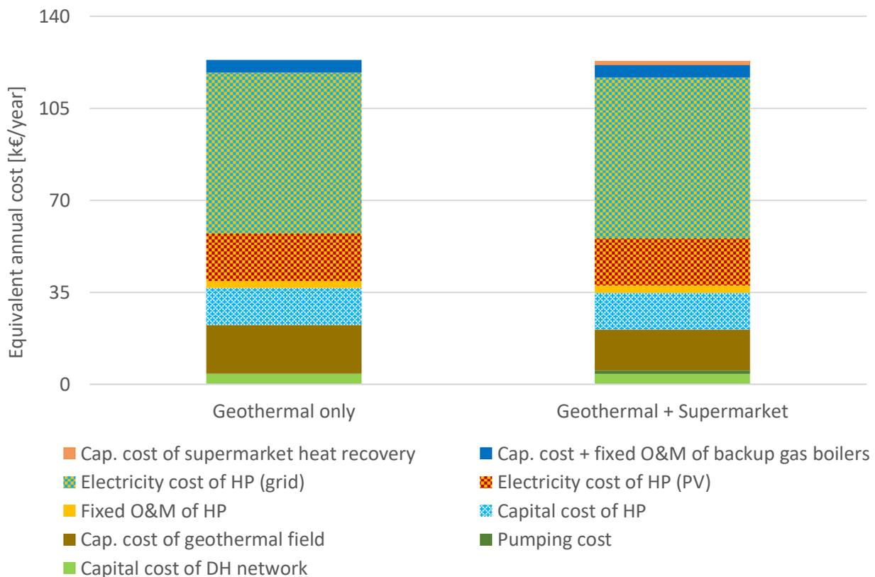
Figure 24: Composition of the equivalent annual cost of the geothermal DH system in Trento.
