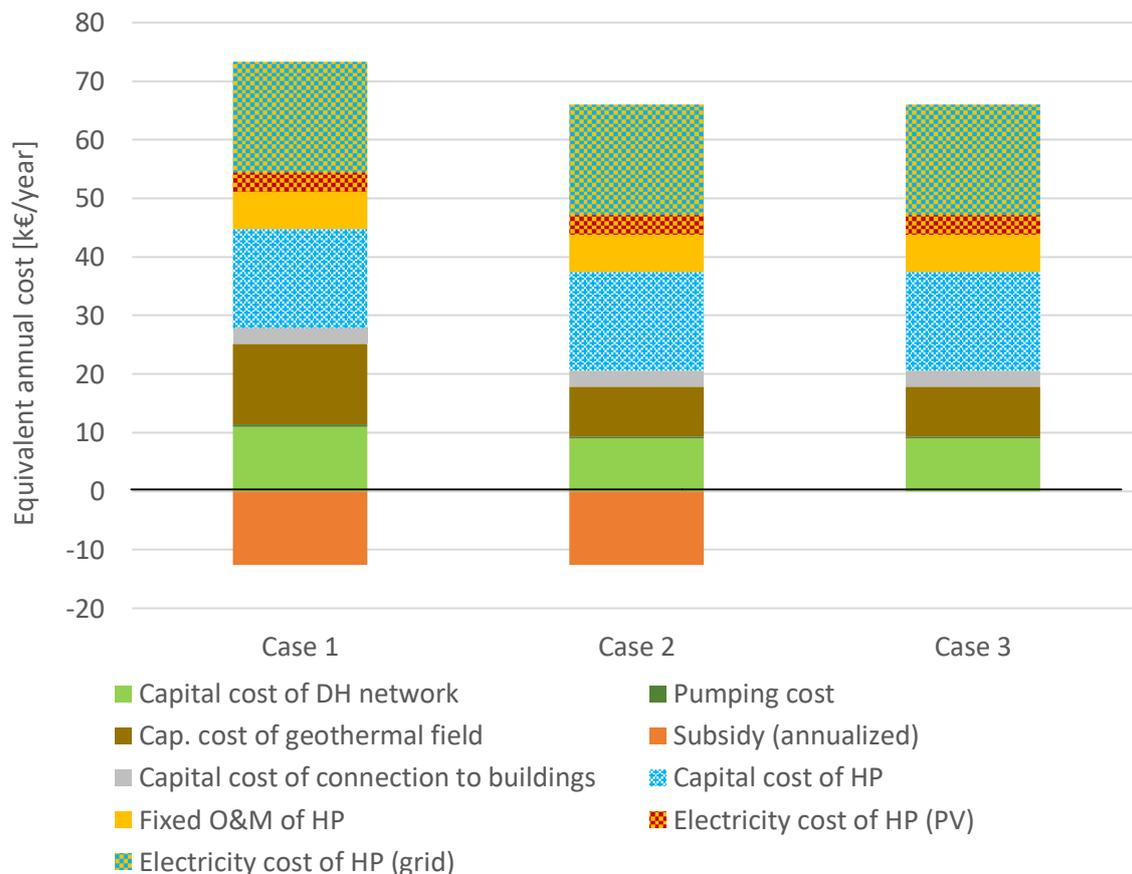
Figure 5: Composition of the equivalent annual cost of the low-depth geothermal DH system in the Cases 1, 2 and 3.
