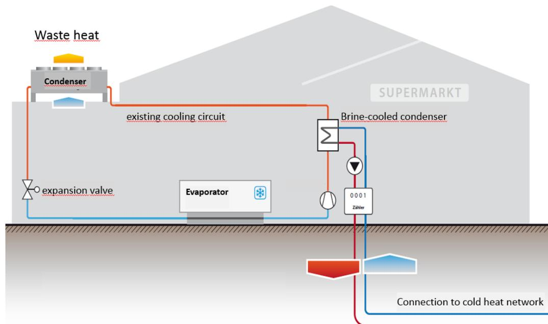
Figure 7. Waste water heat recovery from heat rejection system of the supermarket chillers (Brennenstuhl, 2017).
