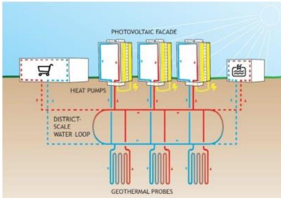
Figure 20: Low temperature smart district heating system to be realized within the Stardust project.
