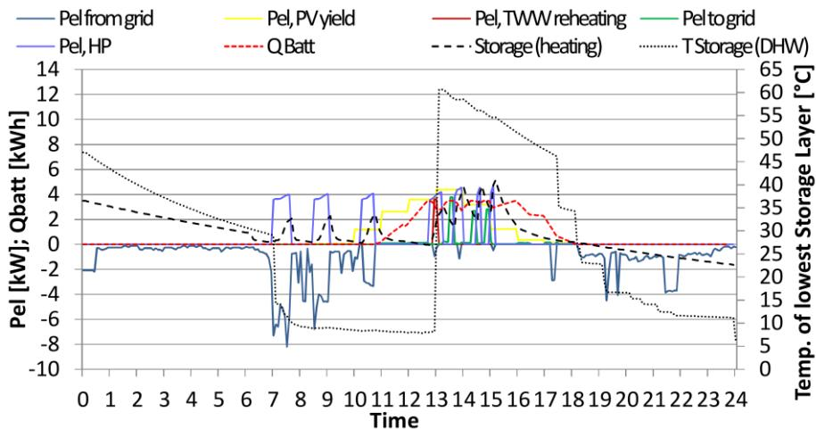
Fig. 9. Heat Pump operation optimized for self-consumption in a residential building (Pietruschka, Brennenstuhl, Matthiss, & Binder, 2015)
