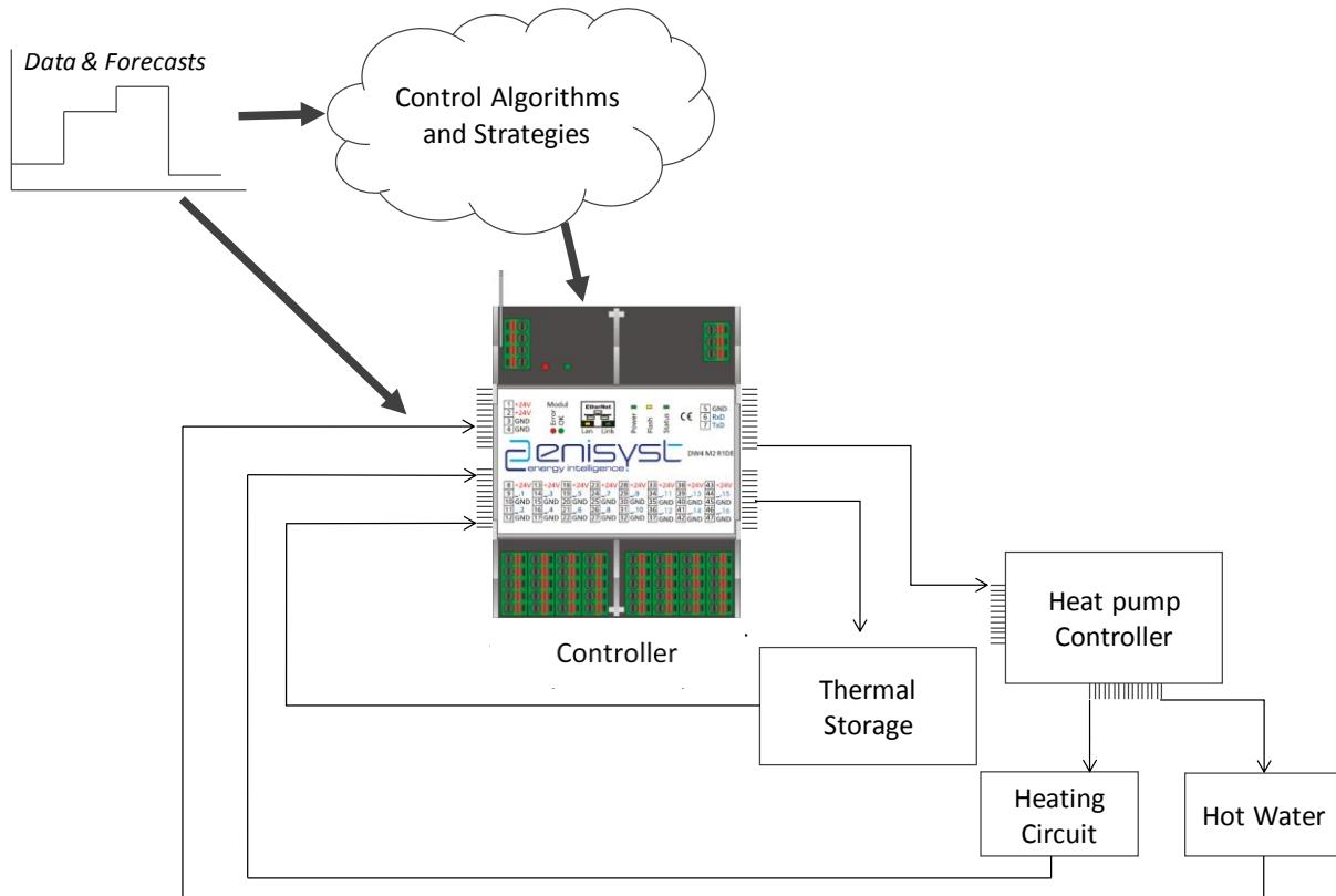
Fig. 1. Control scheme on building level
